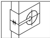
The distance between the edge of the door to the center of the hole is the latch backset. The adjustable latch provides two choices of backsets 2-3/8" (60mm) and 2-3/4" (70mm). Change the backset for the latch according to the illustration.
